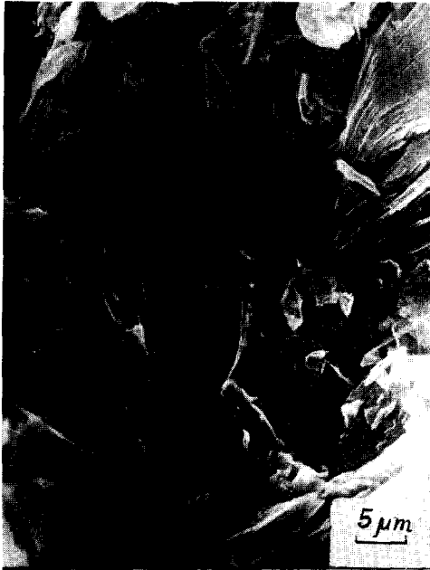
Fig. 1. SEM pictures of high-purity petroleum coke.
